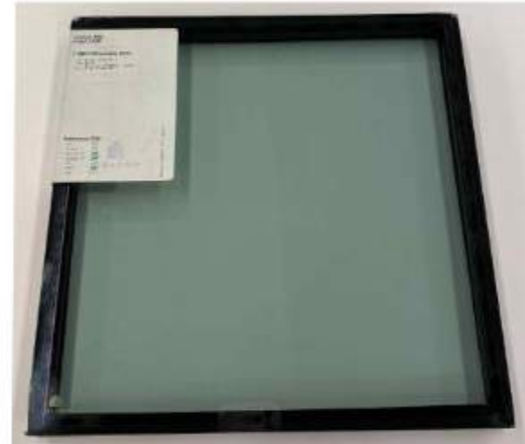
INSULATED VISION GLASS PANELS: - LAMINATED GLASS FOR REGULAR PATIENT ROOMS - LAMINATED GLASS SOUND PATIENT ROOMS - LAMINATED GLASS WITH WARM GRAY SPANDREL
