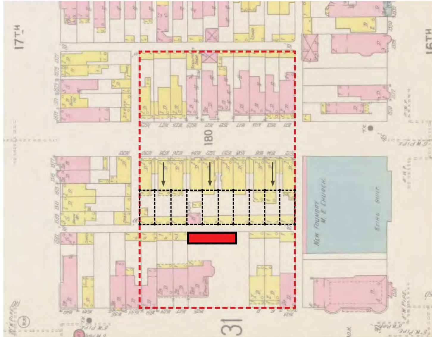
TIGHTEN GRID TOWARDS HISTORIC ALLEY AND EXISTING STRUCTURE, INTERSECTION OF GRID LINES BECOMES COLUMN LOCATIONS
