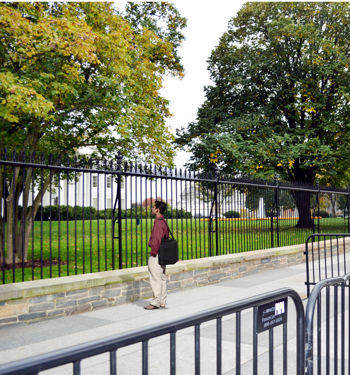
North side along Pennsylvania Avenue Existing (7/8" pickets with 4 5/8" clear space)
