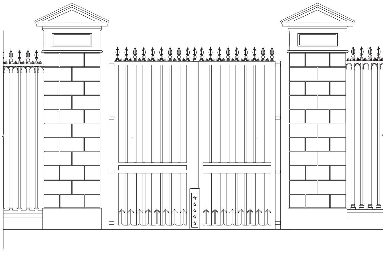
Vehicle Gate Concept: 13'-5" high x 16' wide East & West Executive
