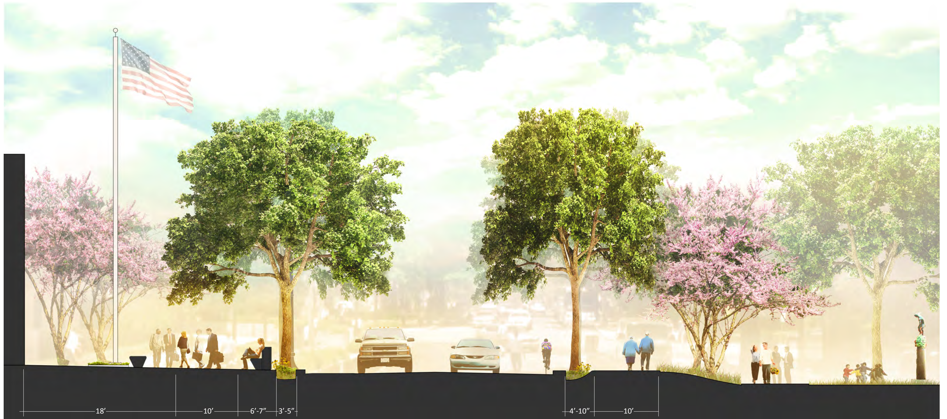
18' 10' 6'-7" 3'-5" 4'-10" 10' Diplomacy Center Plaza Sidewalk Seating Area L.I.D. Planting Area Note: See 5.04 for root zone 21st Street Roadway L.I.D. Planting Area Sidewalk Infill Planting
