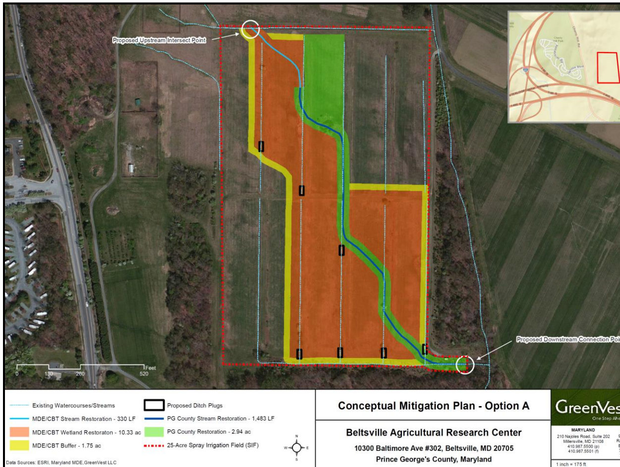
Figure 2. Plan of the 25-acre SIF stream and wetland restoration area (north at left of page).
