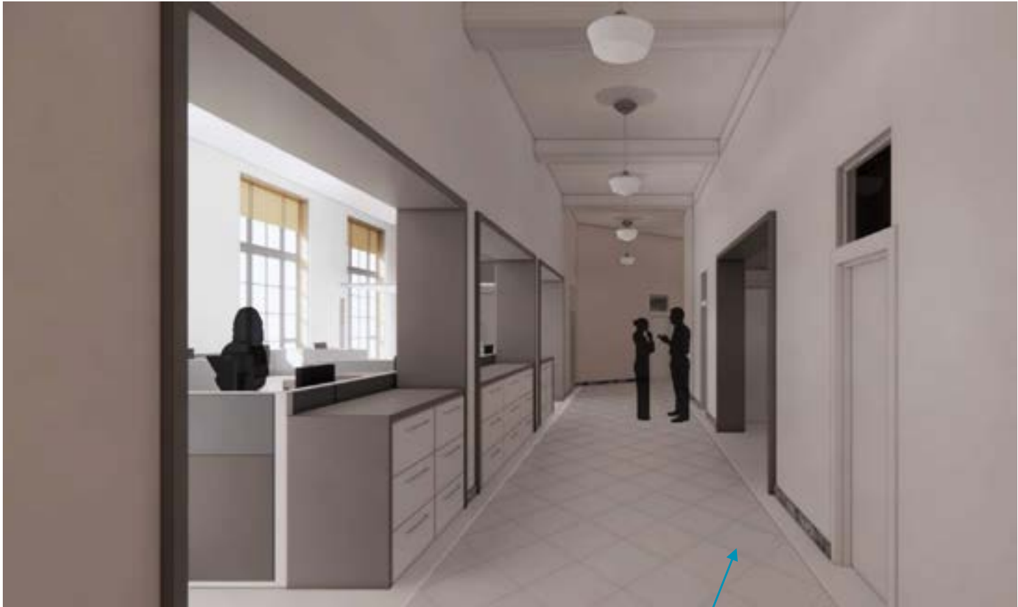
NEW LIGHT WEIGHT CONCRETE TOPPING SLAB AND NEW EPOXY TERRAZZO FLOORING TO MATCH EXISTING PATTERN; NEW COLOR TBD
