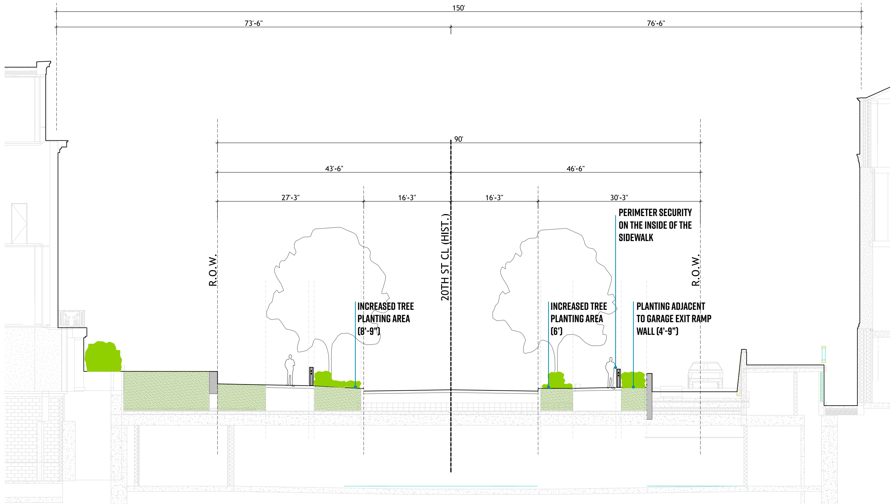
20TH STREET IMPROVEMENTS PROPOSED SITE SECTION - ADJUSTED TO HISTORIC ALIGNMENT | 32'-6" CURB TO CURB
