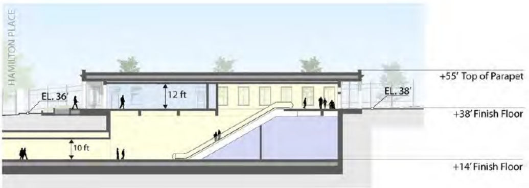
DIAGRAMMATIC SECTION SHOWING THE ABOVE-GRADE SCREENING AND CLEARED VISITOR EGRESS
