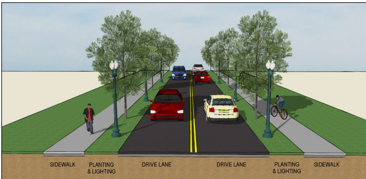
Figure 18 – Secondary Road Streetscape Standards Cross-section
