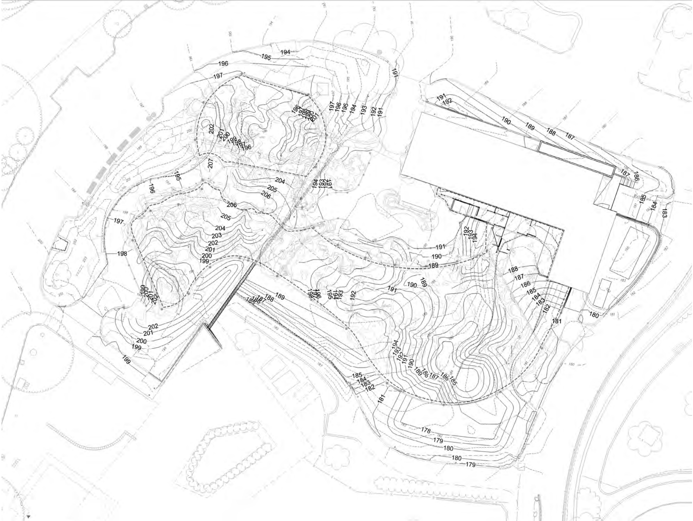
Figure 5.10.2.1: Grading Plan - New Work
