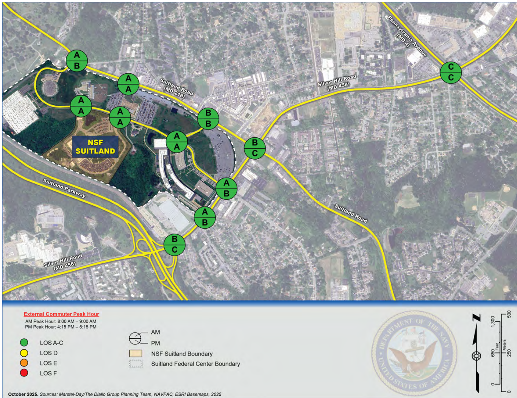
Figure 3.10 Existing (2025) Conditions – Level of Service Summary (HCM Method) (External Commuter Peak Hour)
