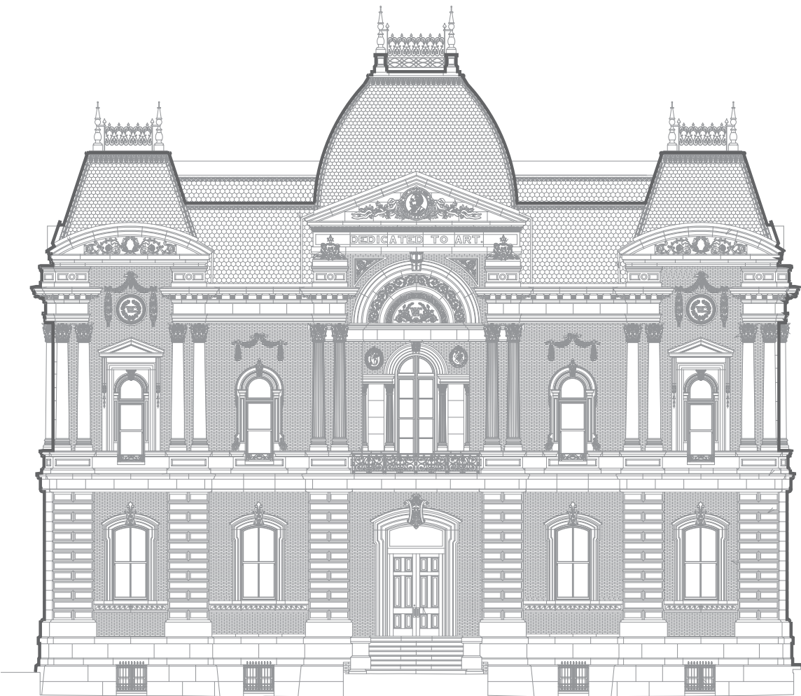
Existing South Elevation showing Non-Historic Window Configuration
