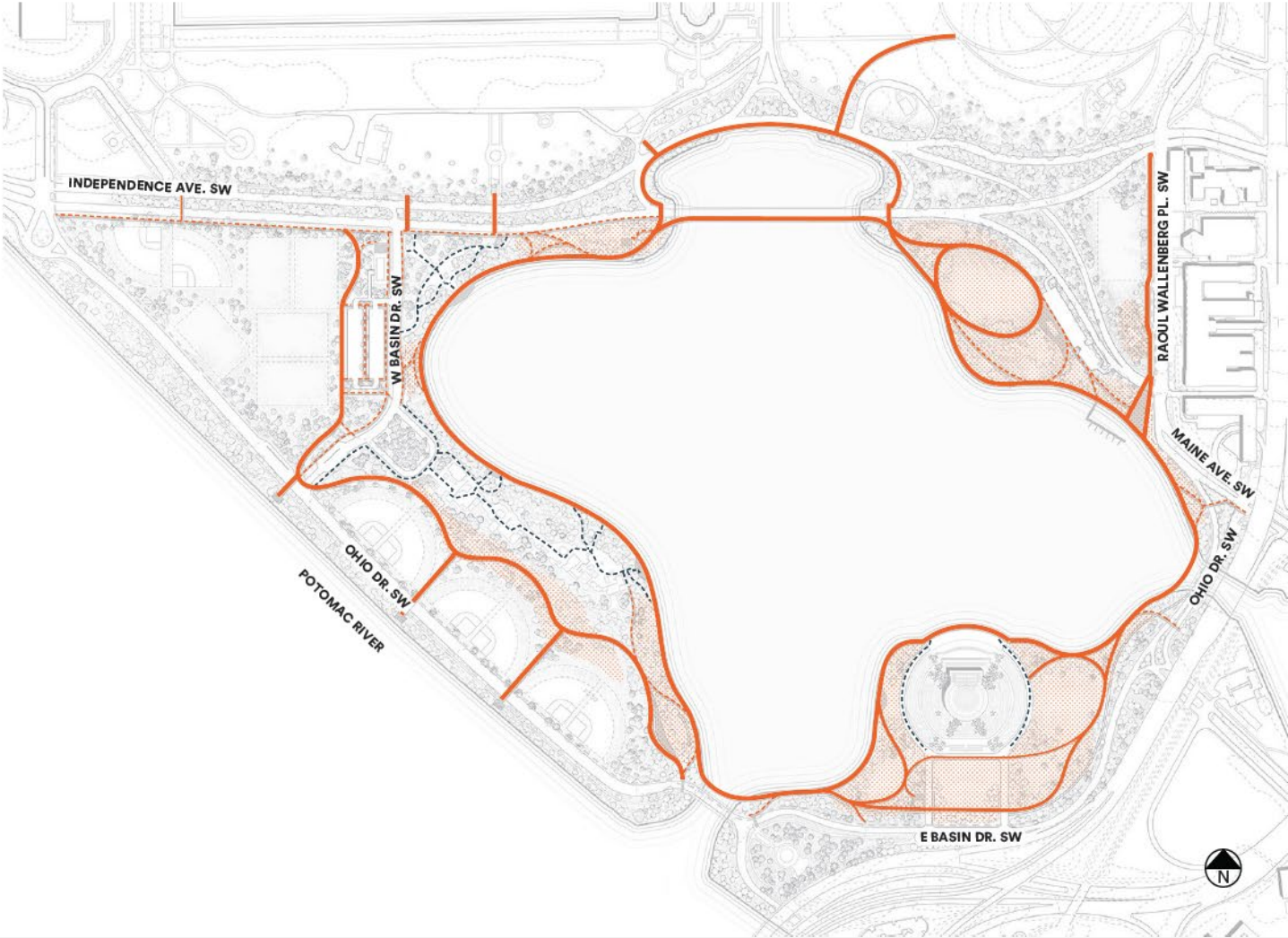
Diagram showing differentiation of 12 ft wide versus 6 ft – 8 ft wide pathways across the site and existing to remain walkways. All pathways are accessible. Open circulation shows zones of free pedestrian movement.
