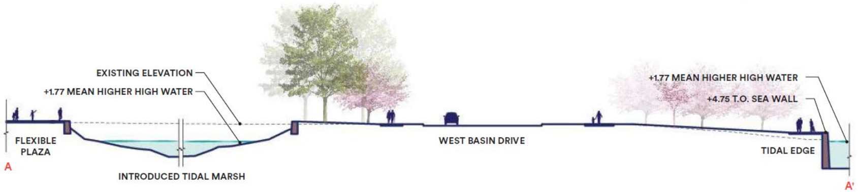
Site section showing transect of interior tidal wetland, flexible plaza, and Tidal Basin edge.
