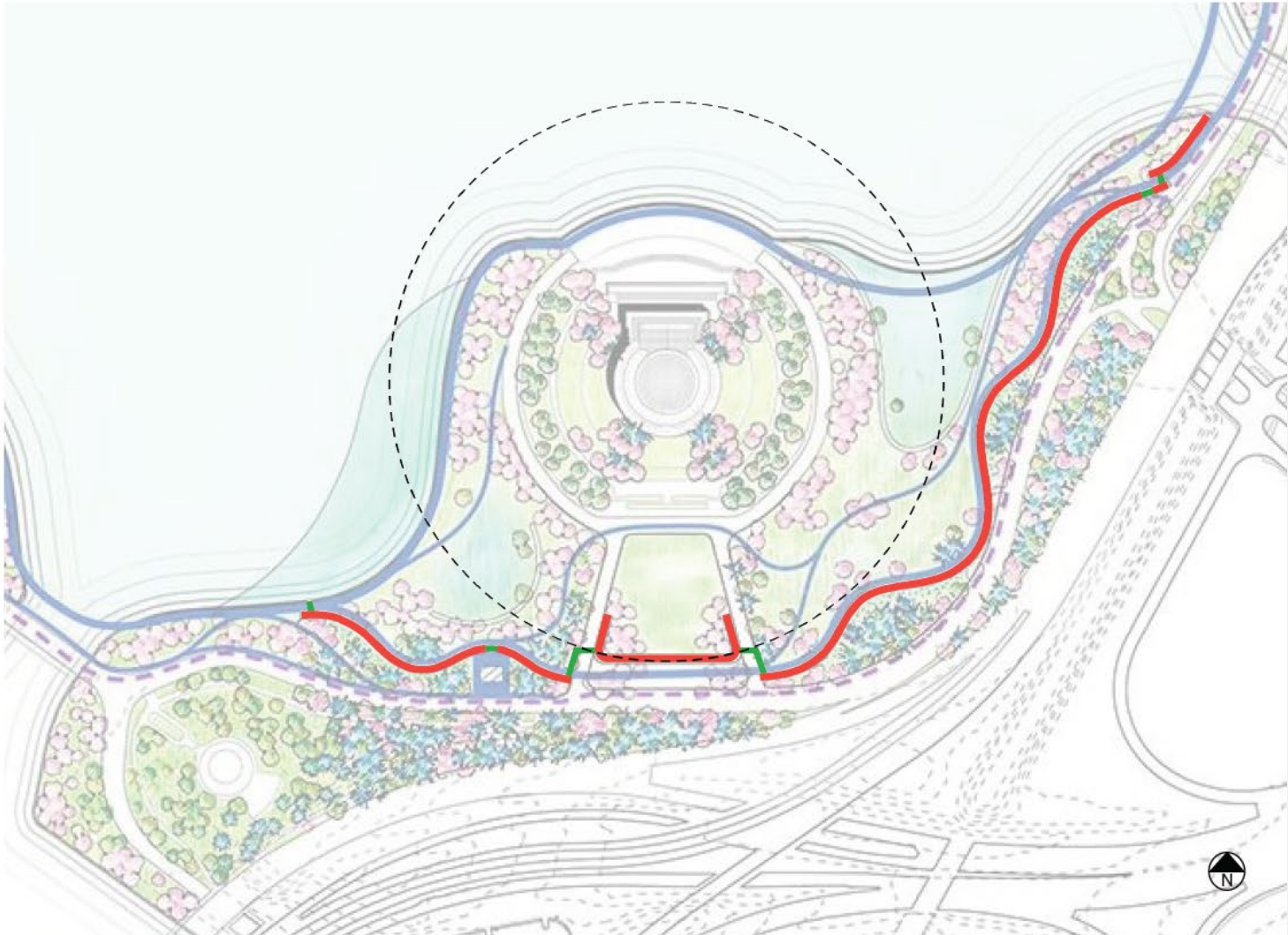
Plan diagram shows area around Jefferson Memorial and includes a proposed security wall, a tapered wall, bollards, and the minimum security setback.
