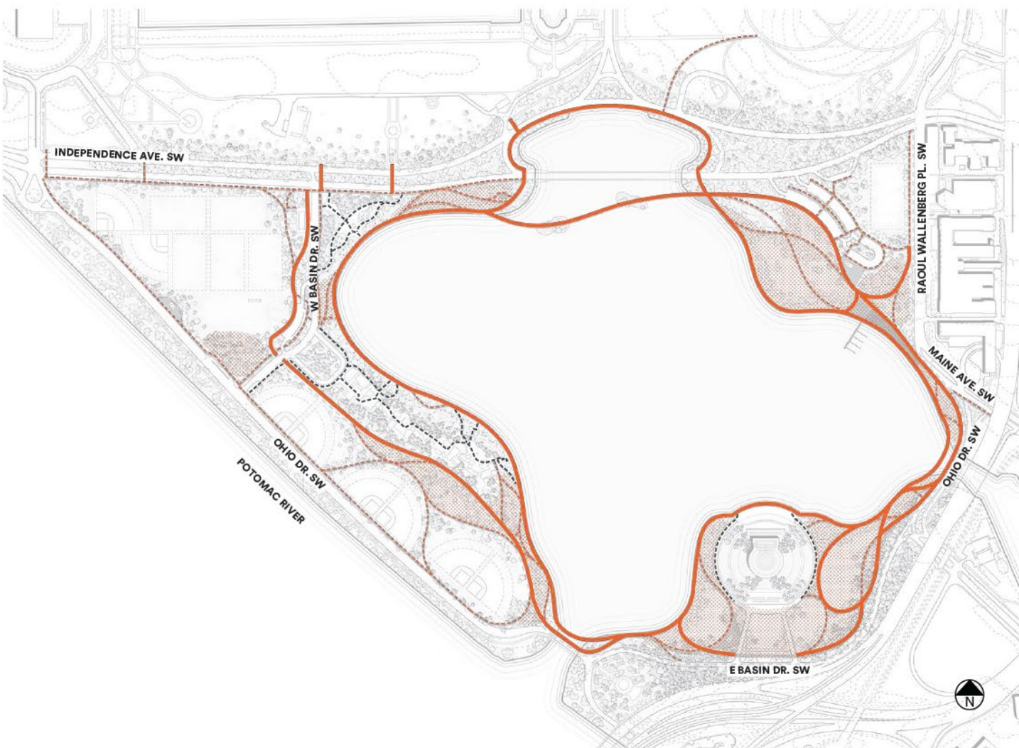
Diagram showing differentiation of 12 ft wide versus 6 ft – 8 ft wide pathways across site and existing pathways to remain. All pathways are accessible. Open circulation shows zones of free pedestrian movement.
