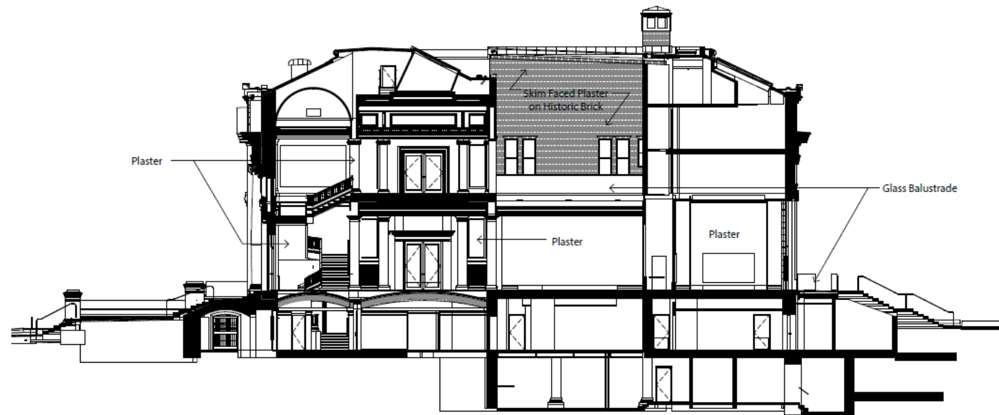
Proposed Transverse Section (Facing West)
