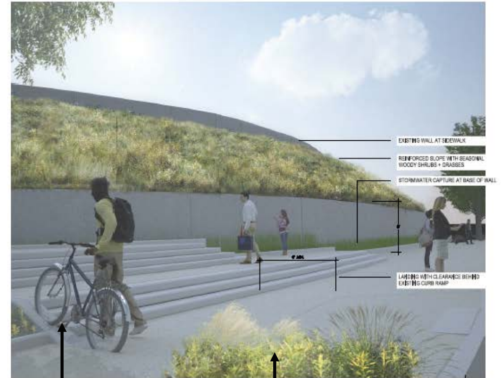
Bike runnel at stairs
