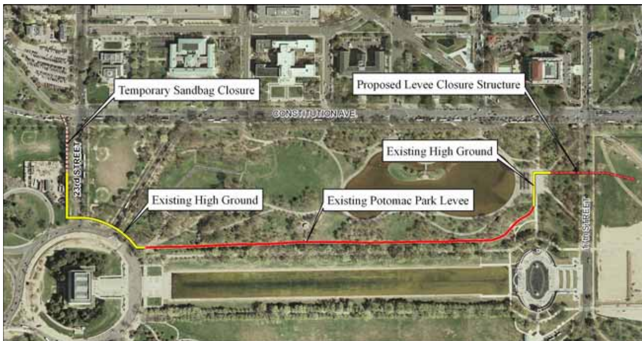
Figure 1. Potomac Park Flood Protection System
