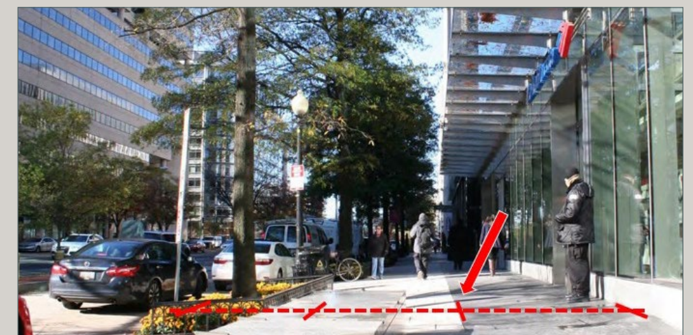
Figure P-7: Example of custom paving extending 1/3 the width of the distance between property line and curb at 18th / K Street NW.
