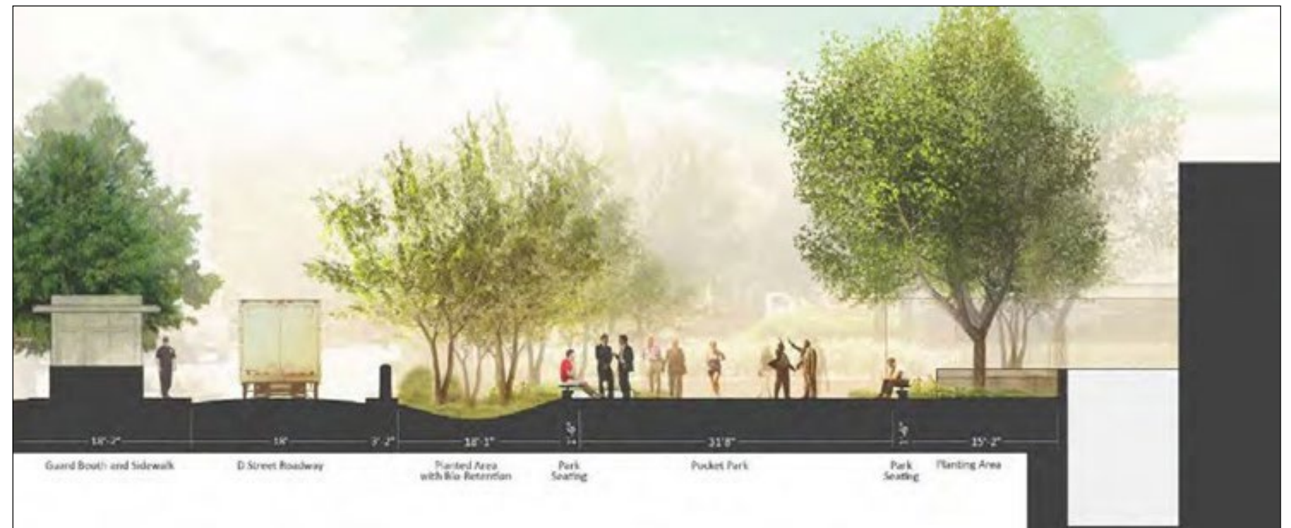
Figure SM-2: Bioretention within a pocket park at the Harry S. Truman Building (Department of State Headquarters) on D Street, NW
