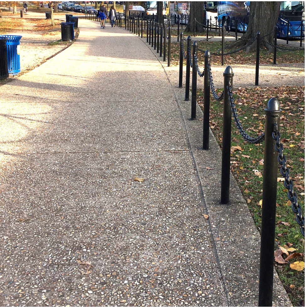
Figure PC-2: Post-and-chain along the pathway protects the root systems of adjacent trees.
