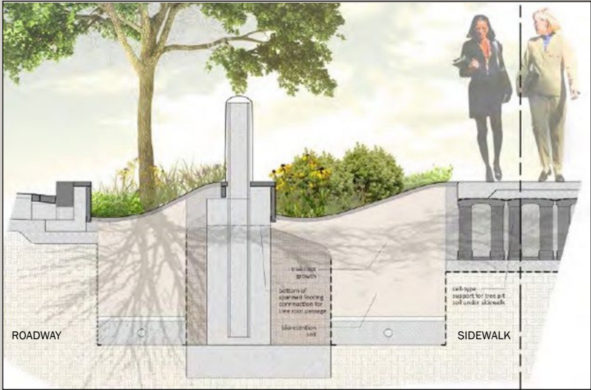
Figure T-6: The Harry S. Truman Building (U.S. Department of State Headquarters) streetscape integrates stormwater management and perimeter security. Non-continuous perimeter security footings, create pathways for enhanced tree root growth.
