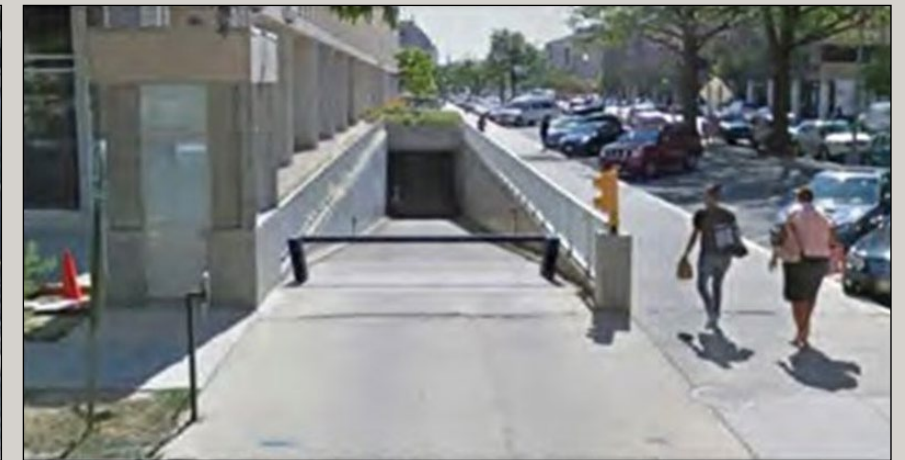
Figure PC-2: Beam barriers are an alternative to more intrusive wedge vehicular barriers and higher-maintenance retractable bollards.
