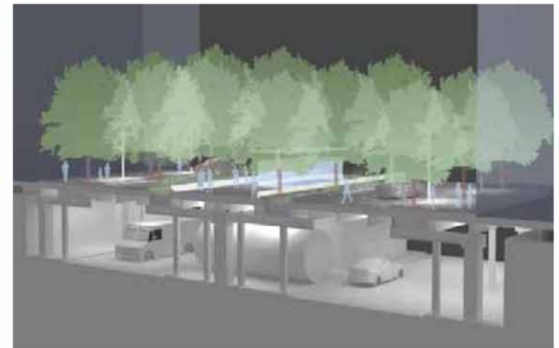
Potential stormwater storage (tank or cistern) under 10th Street
