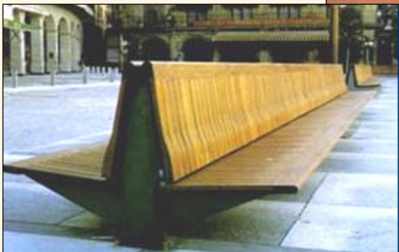
Examples of street furniture that can function as perimeter security after hardening
