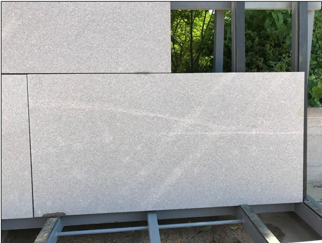
Colonial Rose Granite Mock-up, Sandblast Finish, June 2017.
