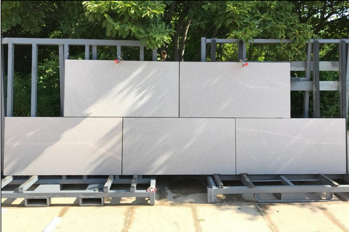
Colonial Rose Granite Mock-up, Sandblast Finish, June 2017.
