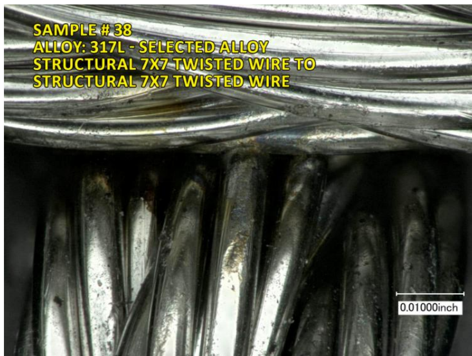
Alloy 317L structural wire weld joint showing no evidence of pitting (~70X magnification).
