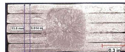
Fig. 4 — A spot weld in a thick assembly, totaling 15.6 mm, is shown. (Photo courtesy of Bombardier.)
