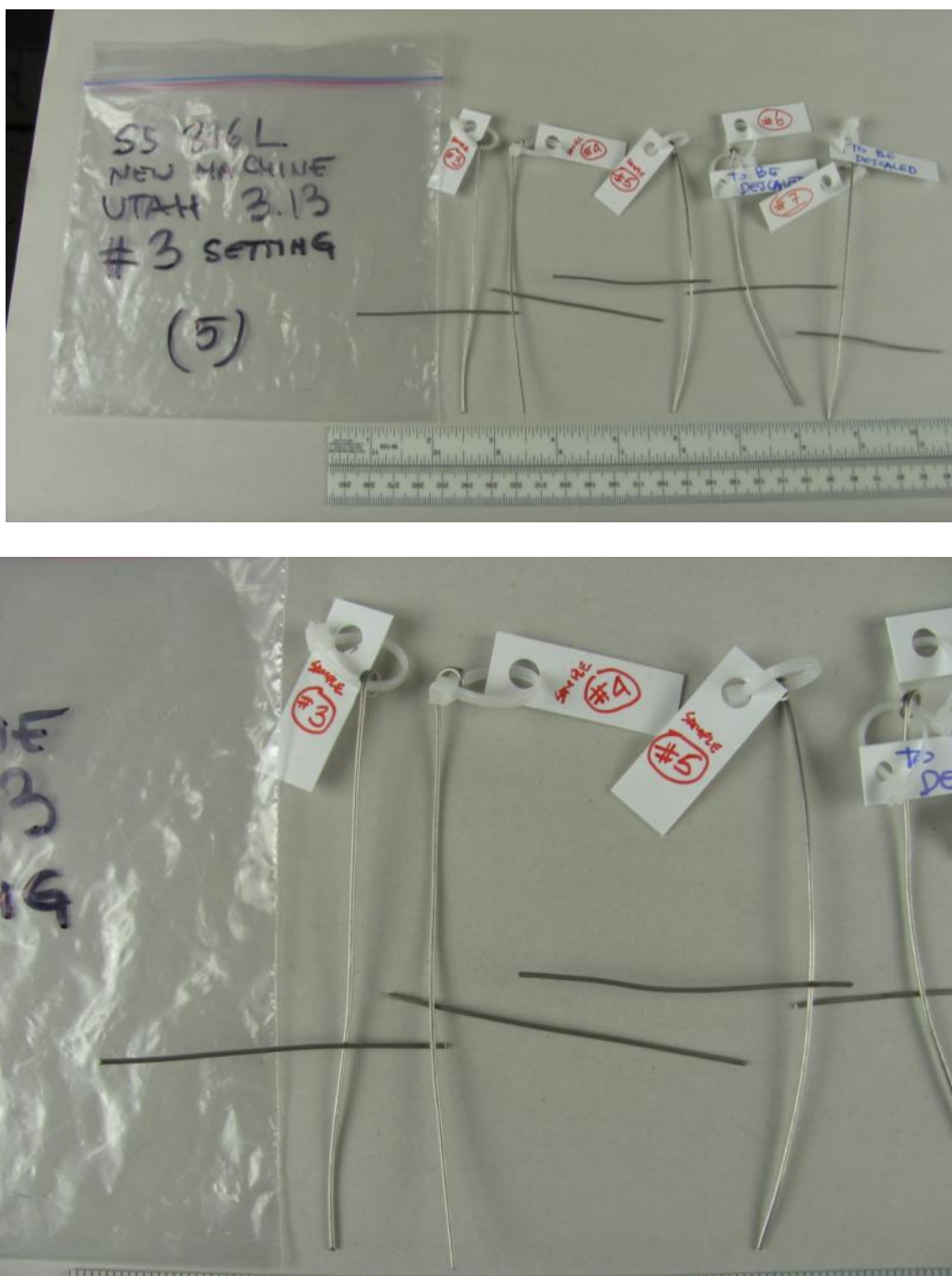
Figure 1 - Macro photographs showing the Type 316L solid wire weld samples submitted for evaluation, as-received prior to descale / passivation and salt spray testing. Samples #3, #4, #5, #6 and #7 are shown.
