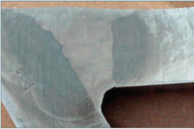
Fig. 9 — Cross-sectional view of welded corner joint. (Courtesy of Mariani Metal, Len Barnes, photographer.)
