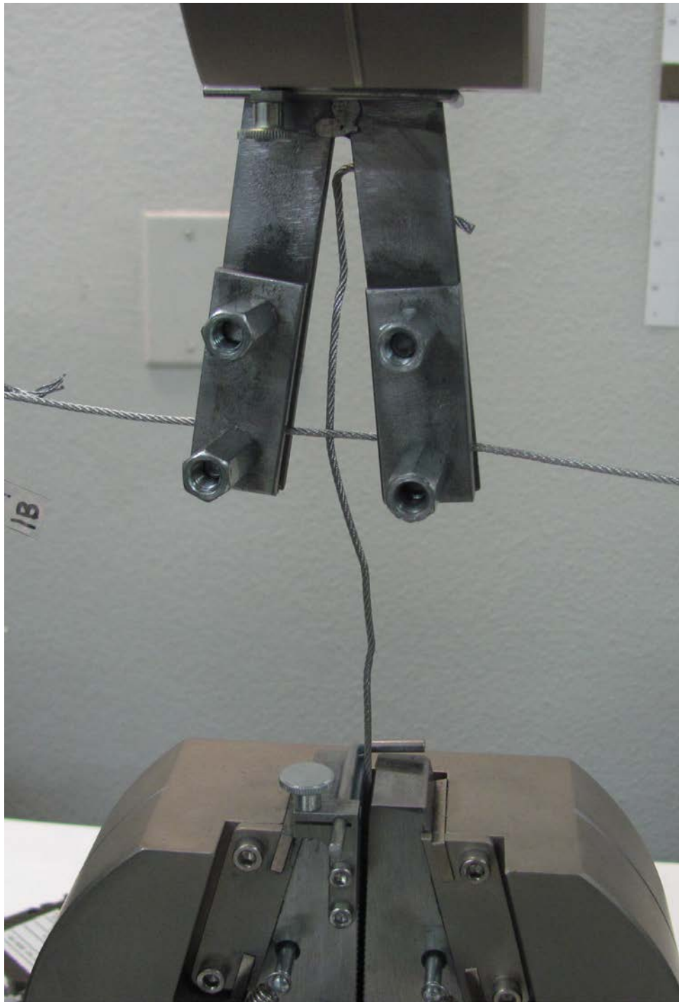
Figure 2 - Macro photograph showing a shear weld strength sample test prior to applying the tensile load.
