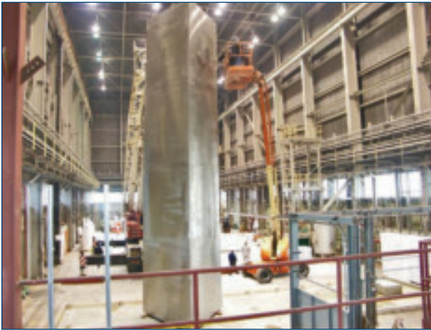
Fig. 11 — The modular section is hoisted for chemical treatments to clean and pickle prior to glass bead blasting. (Photo courtesy of Avesta Welding, LLC, Ron Stahura, photographer.)
