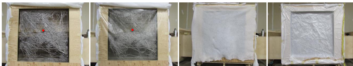
Figure 3: The tapestry sample installed in the pressure chamber. The uncovered tapestry (far left) is covered by three layers; a perforated thin film polymer layer (middle left) and batting breather layer (middle right) are used to minimize the likelihood of the tapestry causing punctures in the thin-film polymer layer (far right).
