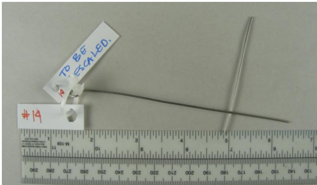
Macro photograph showing Sample #14 made from Type 317L stainless steel shown prior to descale / passivation and salt spray testing.
