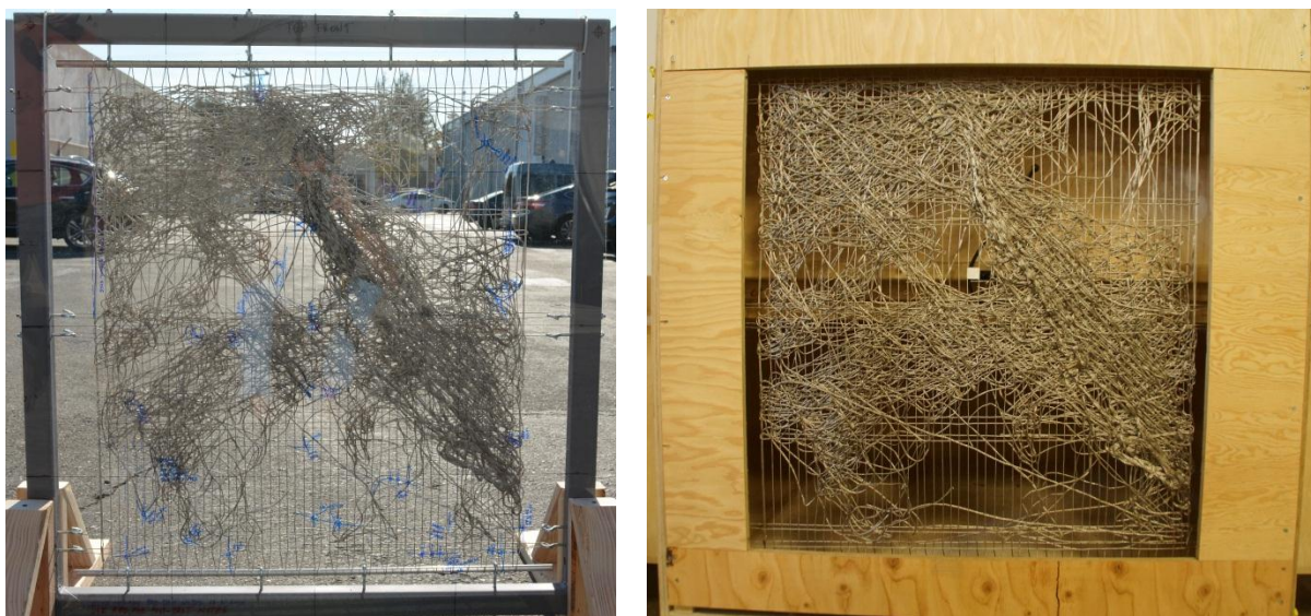
Figure 7: The tapestry sample before (left) and after (right) testing, with a plexiglas sheet indicating deficiencies in the tapestry sample (left only). The markups on the tapestry sample shown in blue were made by the Design Team before testing.
