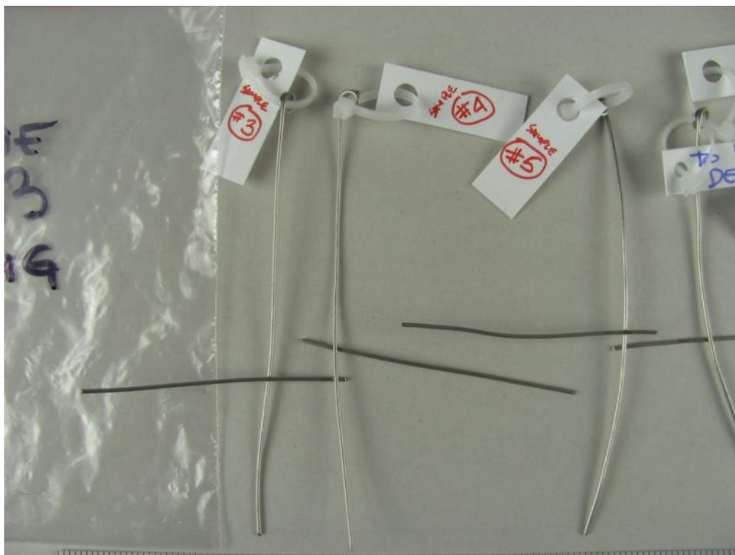
Macro photographs showing the Type 316L solid wire weld samples submitted for evaluation, as-received prior to descale / passivation and salt spray testing. Sample #3, #4, #5, #6 and #7 are shown.
