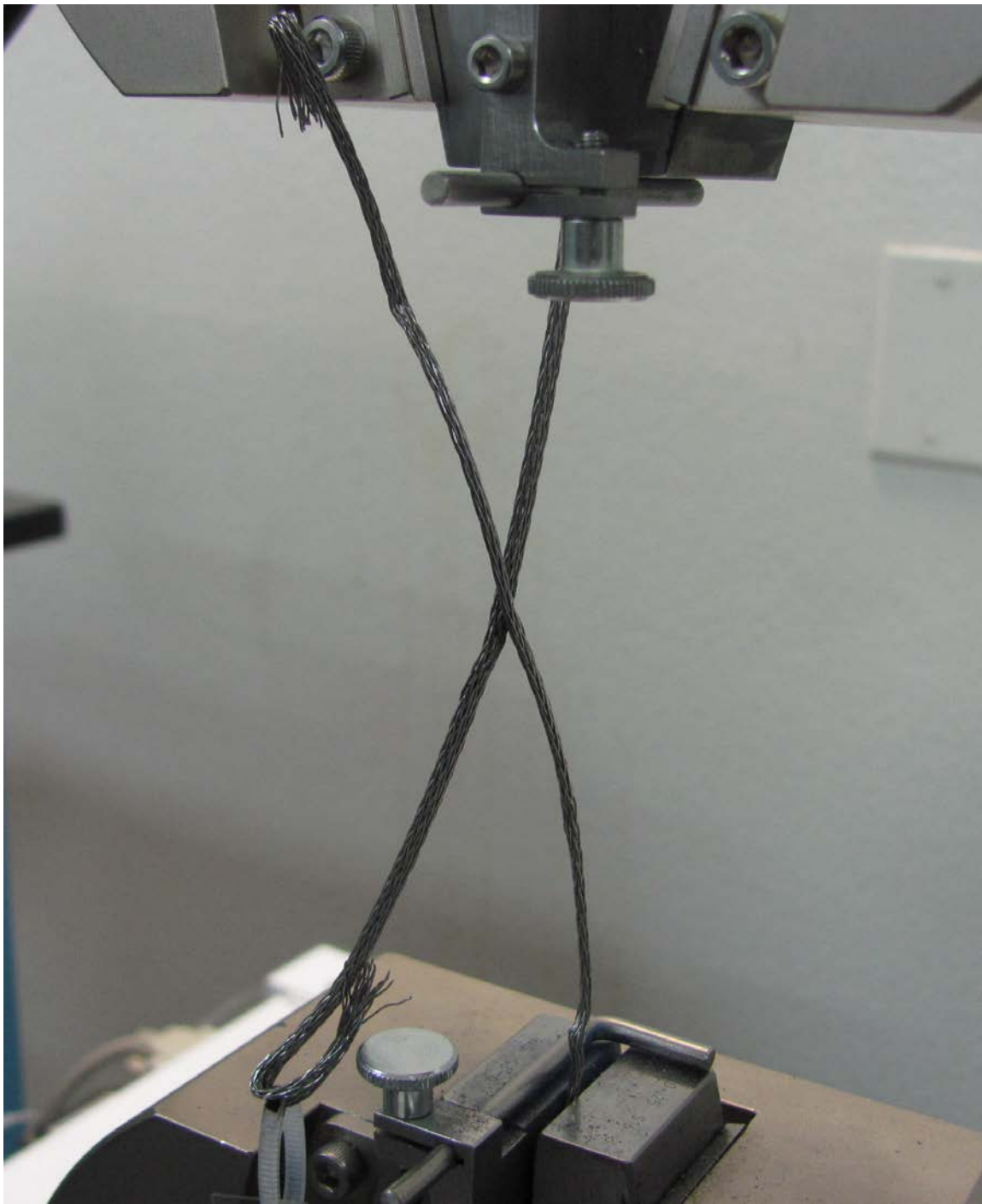
Figure 4 - Macro photograph showing a torque shear weld strength sample during testing.
