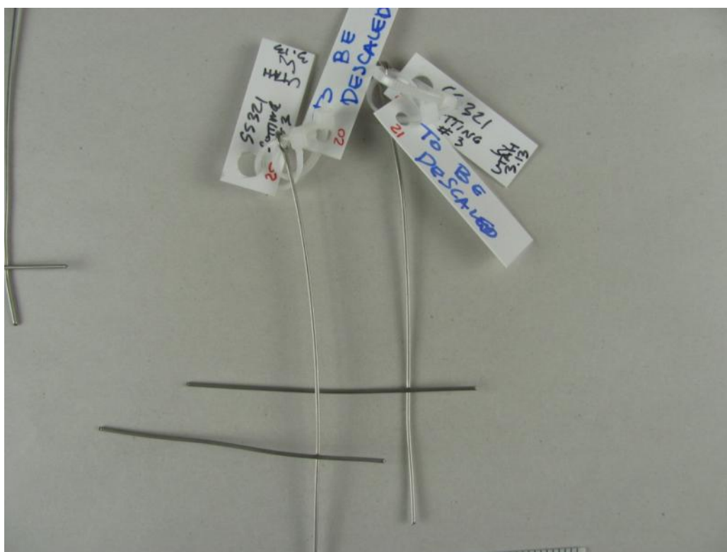
Macro photographs showing the as-received appearance of the Type 321 solid wire weld samples prior to descale /passivation and salt spray testing. Sample # 17, #18, #19, #20 and #21 are shown.
