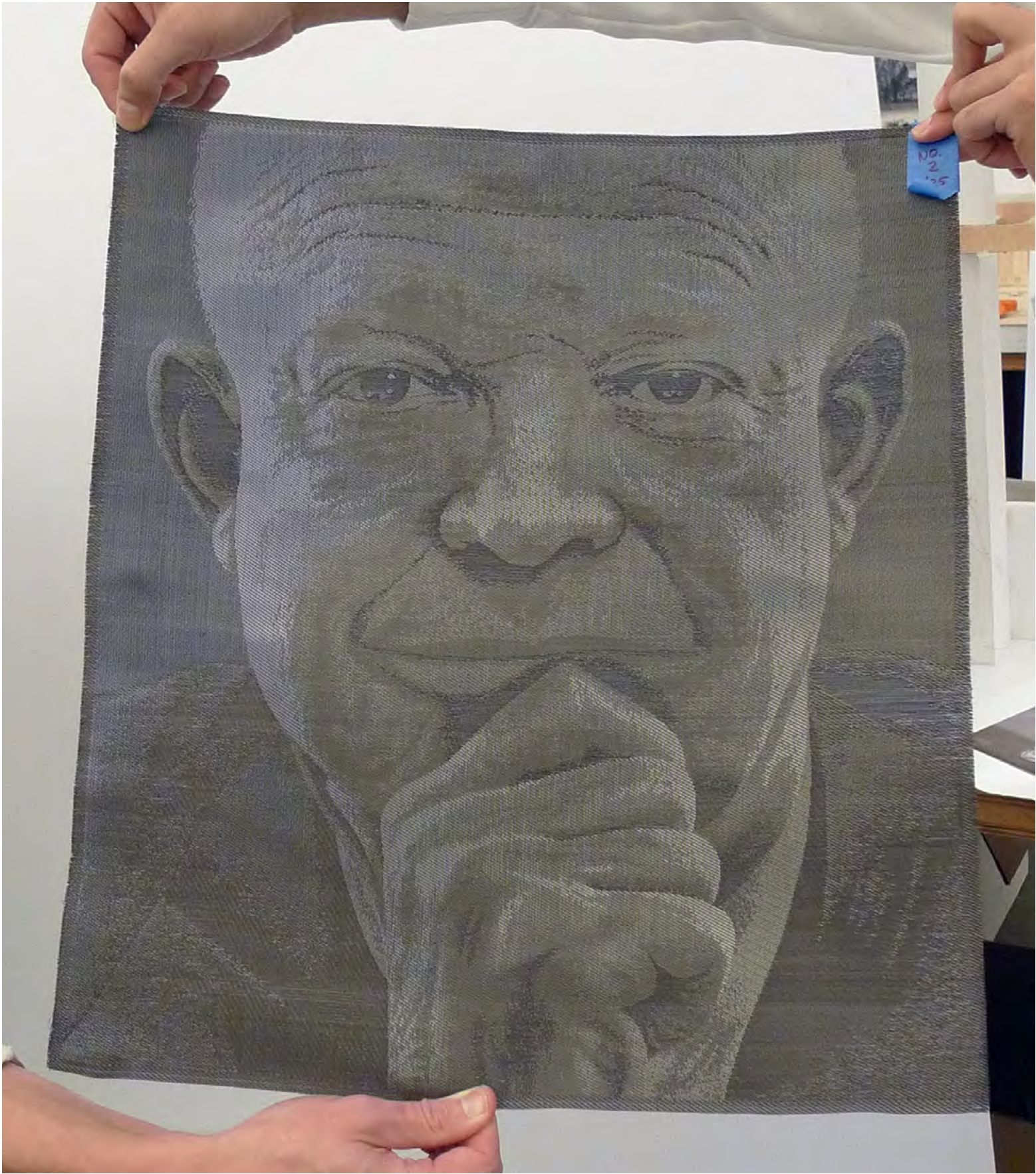
JACQUARD WOVEN SAMPLE WITH VERTICAL STAINLESS STEEL WIRE AND HORIZONTAL BLACK COATED COPPER WIRE
