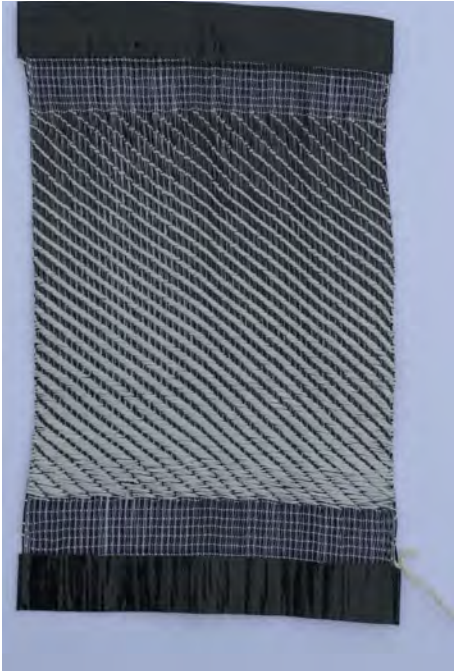
WEAVE STRUCTURE SAMPLE WITH PTFB (TEFLON)
