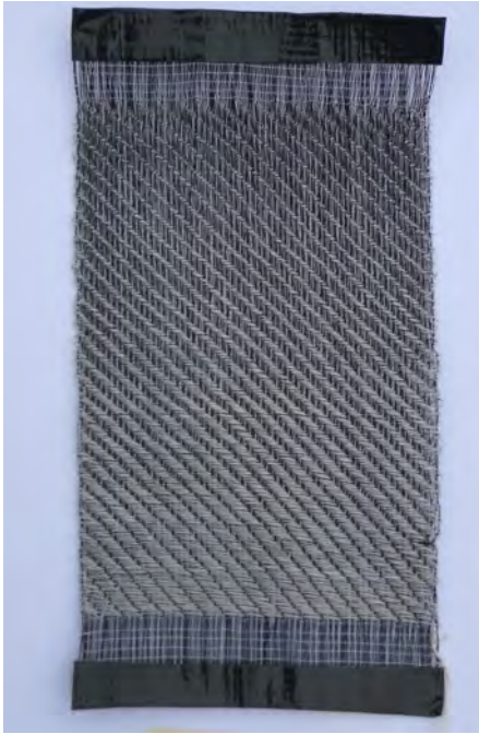
WEAVE STRUCTURE SAMPLE WITH STAINLESS STEEL WIRE & BLACK WIRE
