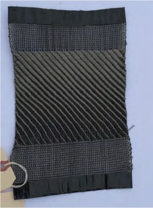
WEAVE STRUCTURE SAMPLE WITH STAINLESS STEEL YARN
